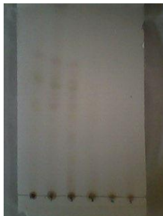
Plate 4. Chromatogram of column fractions in hexane/ethyl acetate (8:2) after spray with 20% sulphuric acid and heated at 105°C for 15 min.
